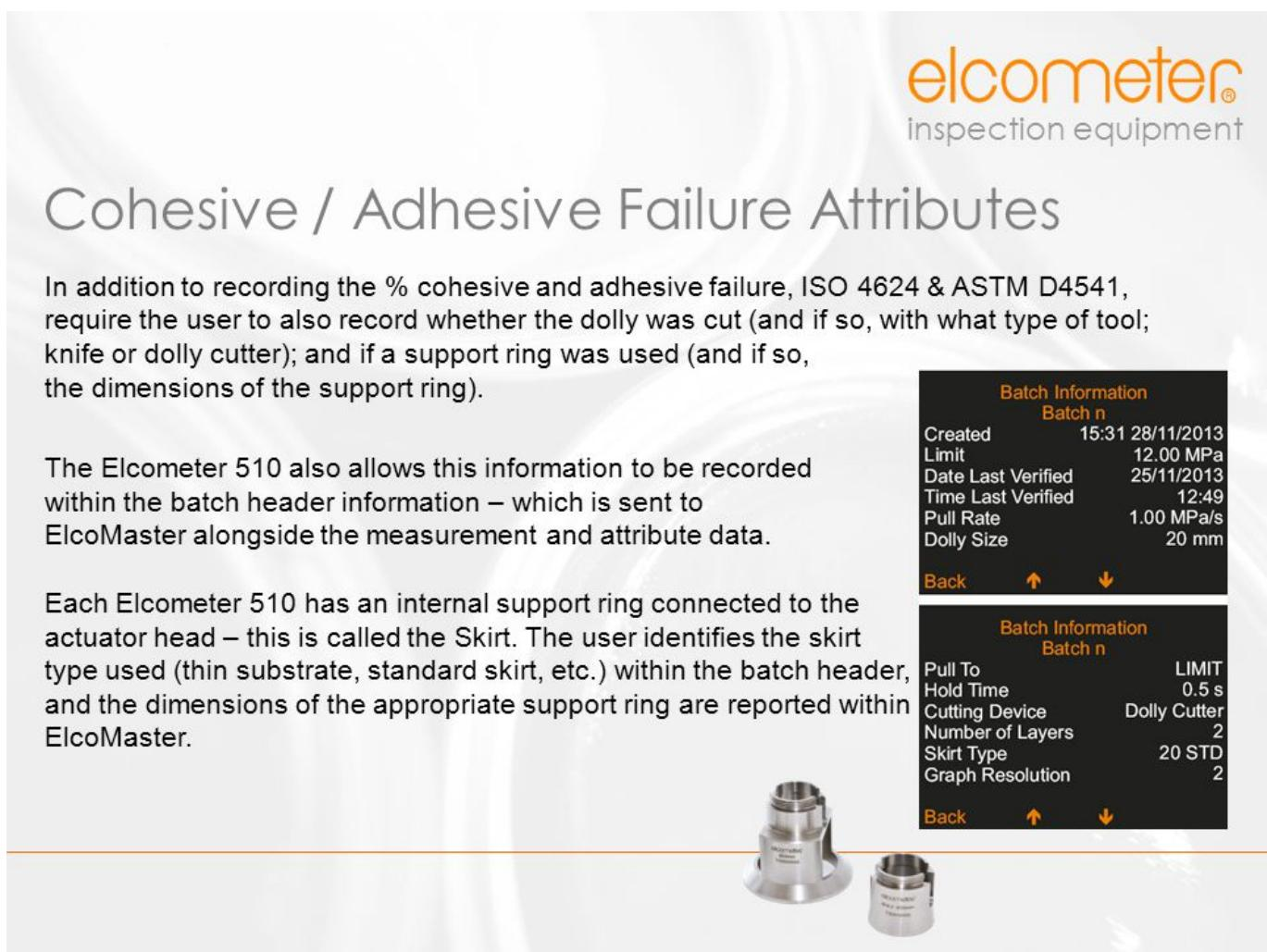
The Elcometer 510 also allows this information to be recorded within the batch header information – which is sent to ElcoMaster alongside the measurement and attribute data.
